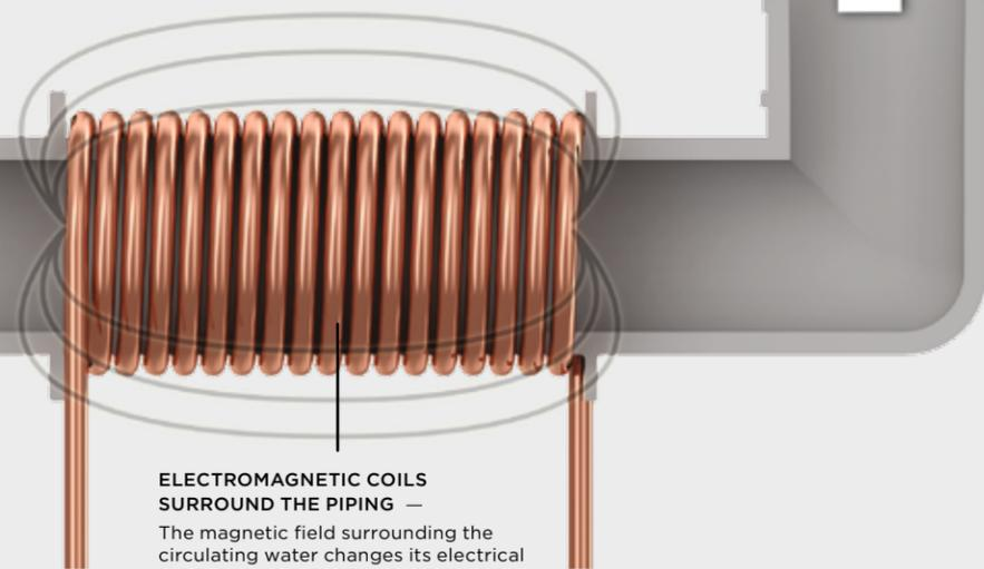
**ELECTROMAGNETIC COILS SURROUND THE PIPING** — The magnetic field surrounding the circulating water changes its electrical and chemical characteristics.
